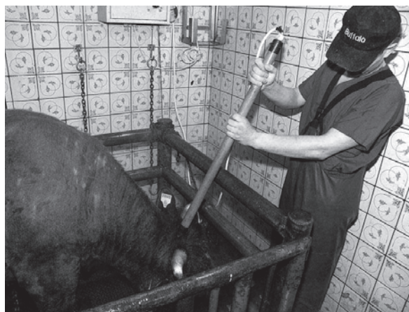
Photo 2 - Inadequate stunning equipment for cattle. The current from a single electrode passes through the body of the animal rather than spanning the brain.
