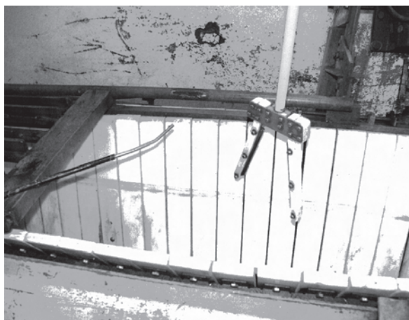
Fotografía 5. Electrical stunning with two points application
